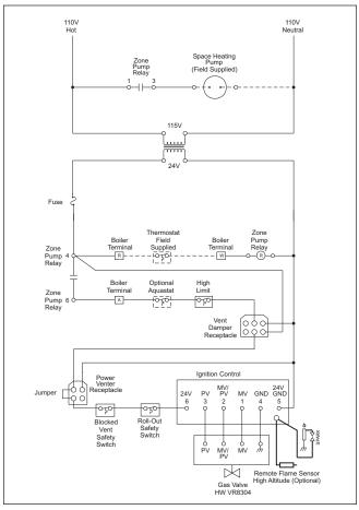
Figure 9b. Schematic, Spark Ignition System (BJVS 50 & 75).
